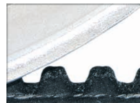
Special belt for exceptionally quiet, non-slip measuring.
