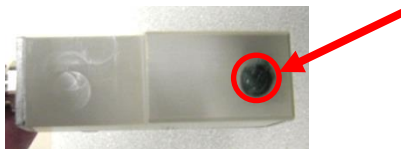
Figure 11: Transducer with an approx. peanut-sized drop of coupling gel
