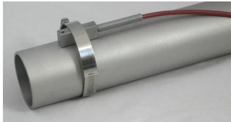
Figure 22: At pipe mounted Pt100
