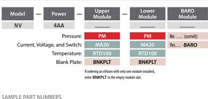
NV-4AA-3BAR-300BAR-BARO nVision with 3 bar pressure module (upper) and 300 bar pressure module (lower); and a BARO module option.
