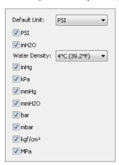
Use the Unit button options to control which units the pressure gauge will display.
