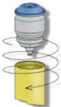
Installing Piston-Cylinder Module
